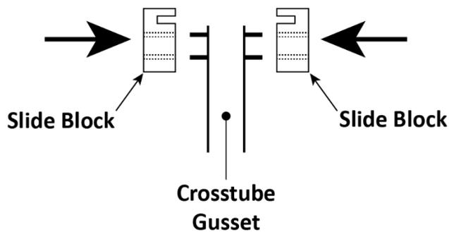
The four Slide Blocks on a Gusset, when put into place, create two Slots about four inches wide and half an inch deep. There is one Slot at the top of the Gusset and a second Slot at the bottom; the Ladder **must** go through **both** Slots on the Gusset.
