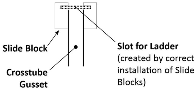
3. Using a Forklift or Shop Crane, raise the Crosstube with the Slide Blocks installed above the top of the two Posts that it goes between, lower it to just over the top of the Post, orient the Slide Blocks over the openings in the Posts, then slide the Crosstube down.
