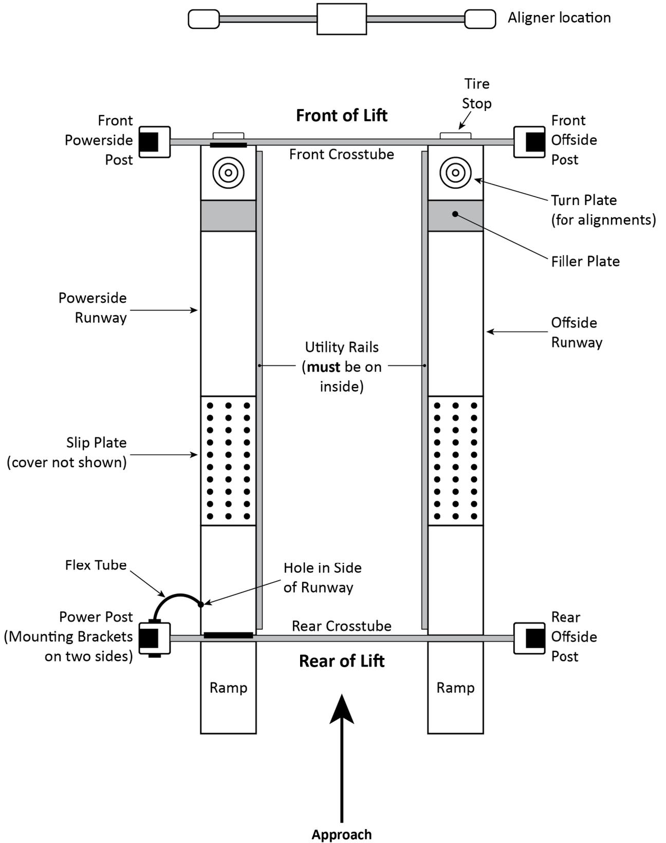
Drawing not necessarily to scale. Some components not shown. Aligner is a separate product; it is not included with the Lift. The Front of the Lift is the end **opposite** the Ramps.
