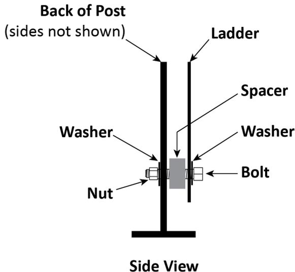
2. Put a Washer next to the Bolt head, then insert the Bolt just through the elongated hole near the bottom of the Ladder.
