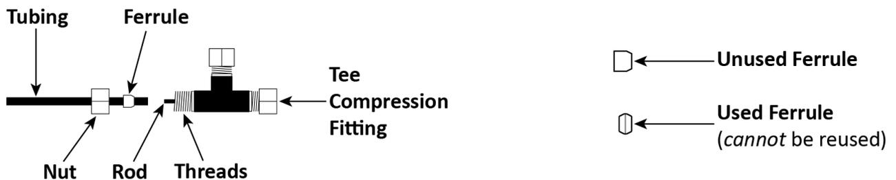
**Important:** *Ferrules can only be tightened once.* When you tighten the Nut on the Threads, the Ferrule gets compressed; it literally changes shape and **cannot** be used again.
