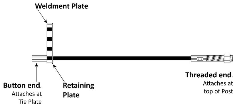
*Drawing not to scale. Not all components shown. The Weldment Plate, located under the Powerside Runway, comes attached to the end of the Piston on the Hydraulic Cylinder.*
