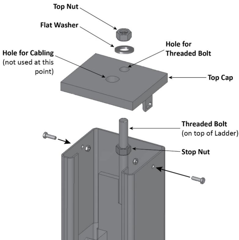
4. Put a Top Cap onto the top of the Post, securing it on the sides with one Hex Head Bolt and one Nyloc Nut on each side of the Top Cap.
