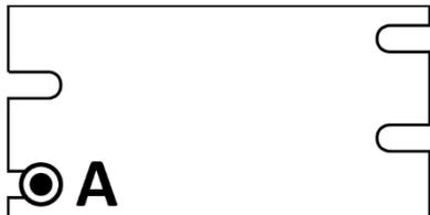
Drawing shows Button end of Cable A in its slot on the Weldment Plate.
