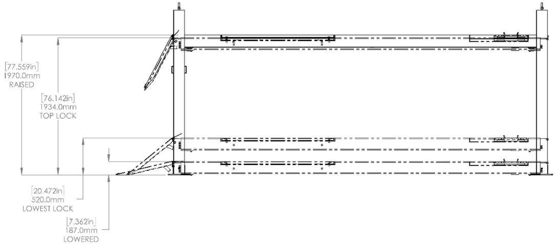
1. DIMENSIONS SHOWN ARE WITH THE LOCK LADDERS ADJUSTED ALL THE WAY UP
