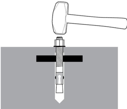
The Expansion Sleeve of the Anchor Bolt may prevent the Anchor Bolt from passing through the hole in the Base Plate; this is normal. Use a hammer or mallet to get the Expansion Sleeve through the Base Plate and into the hole.
