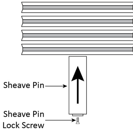
*Using a Red Lithium Grease Lubricate each Sheave Pin Prior to inserting through the Sheaves. Figure shows Sheave Pin being pushed up into the four Cable Sheaves at the Rear of the Lift.*
