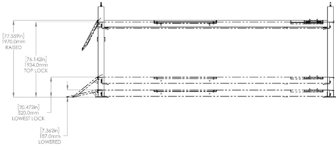
1. DIMENSIONS SHOWN ARE WITH THE LOCK LADDERS ADJUSTED ALL THE WAY UP
