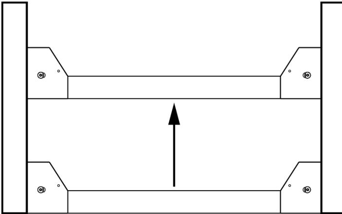
**Important:** The Slack Safeties cannot be engaged as you continue with the installation. Because the Cables are not in place yet, the Slack Safeties are going to engage when you manually raise the Crosstubes. You need to disengage them after you have raised the Crosstubes. The Primary Safeties are not impacted; they will engage normally when you manually raise each Crosstube, which is what you want.
