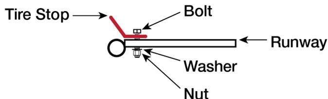
**Note:** Make sure to orient the Tire Stop so that it is sloping away from the Runways. This creates an angle best suited to holding the Tire in place.
