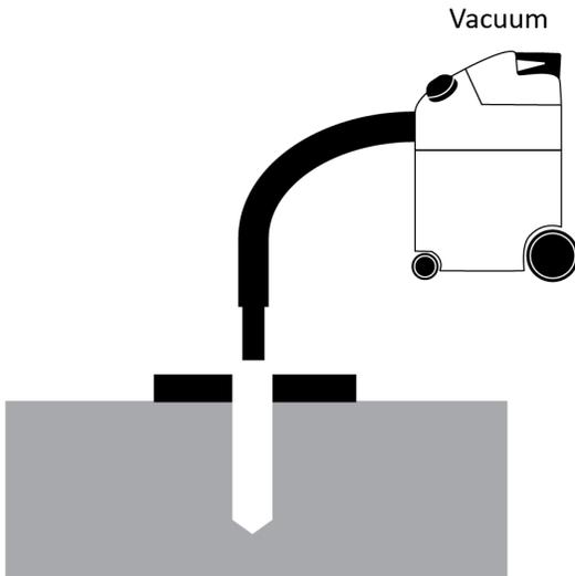
BendPak recommends using a vacuum to get the hole very clean. You can also use a wire brush, hand pump, or compressed air; just **make sure to thoroughly clean each hole**.
