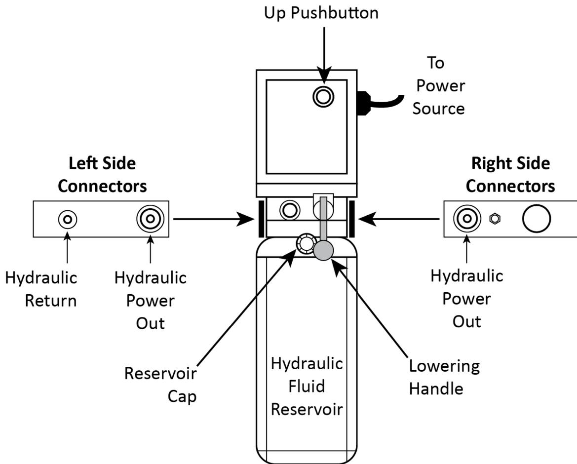
**Note:** The Up Pushbutton for Power Unit 1 is centered; it is off-center to the right on Power Unit 2.
