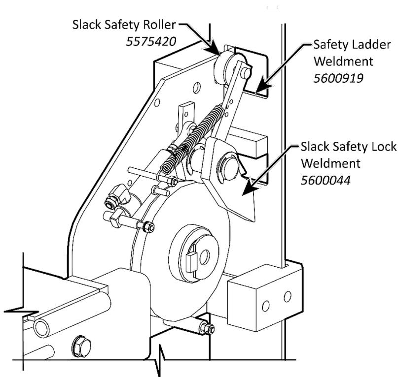
Figure not to scale. Components removed for clarity.
