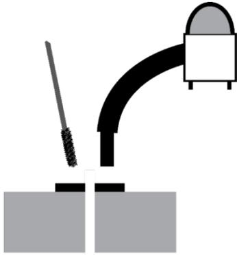
BendPak recommends using a vacuum to get the hole very clean. You can also use a wire brush, hand pump, or compressed air; just **make sure to thoroughly clean each hole.**
