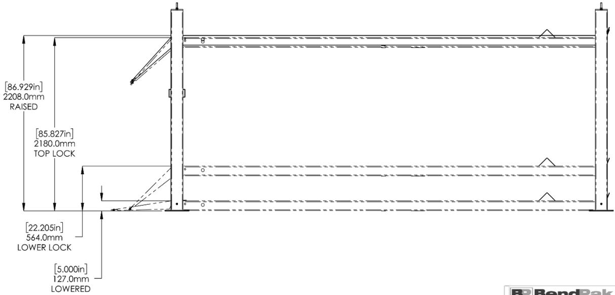
1. DIMENSIONS SHOWN ARE WITH THE LOCK LADDERS ADJUSTED ALL THE WAY UP
