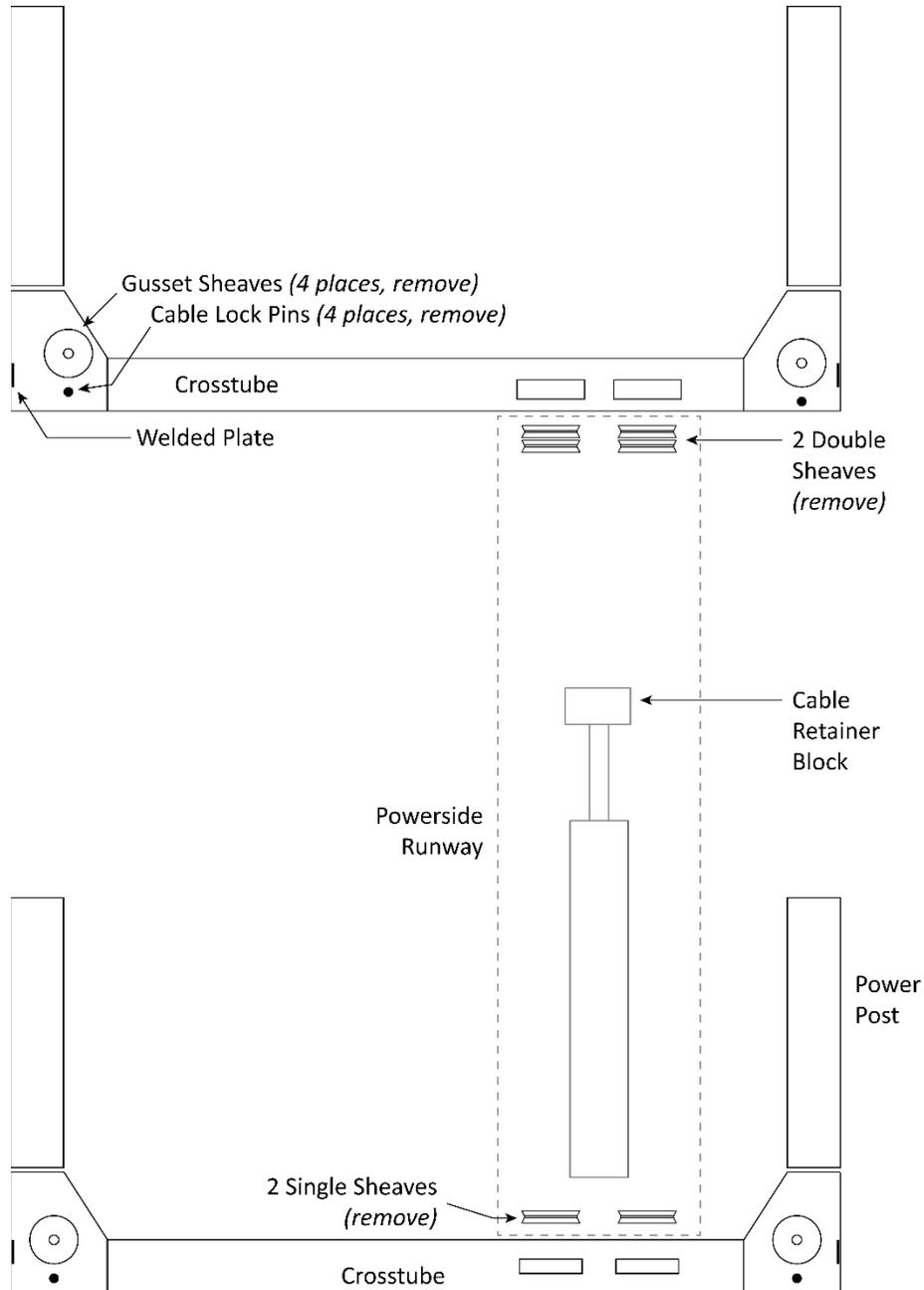
*Not to scale. Components removed for clarity. Combines top and side views.*
