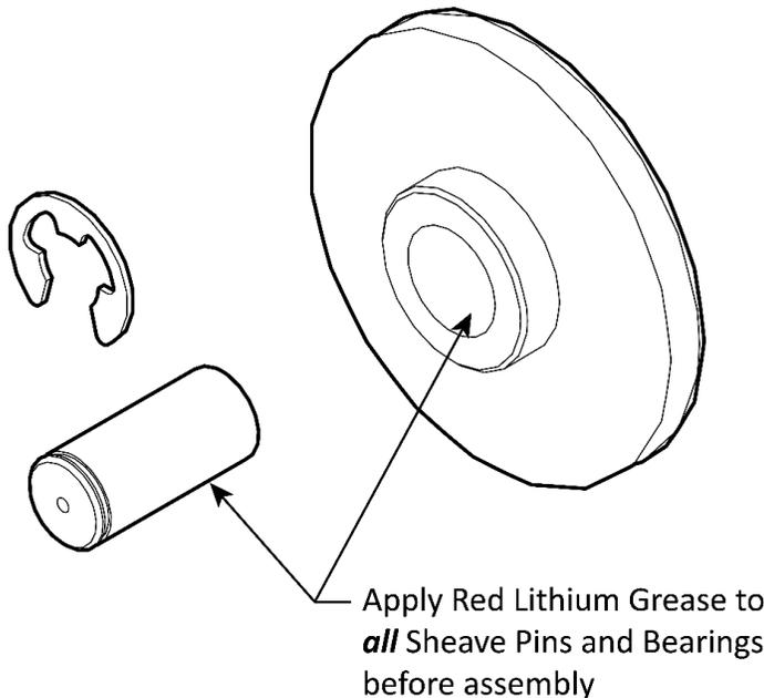
5. With the Lifting Cable in place, reinstall the Gusset Sheave and the Cable Lock Pin in Post A.
