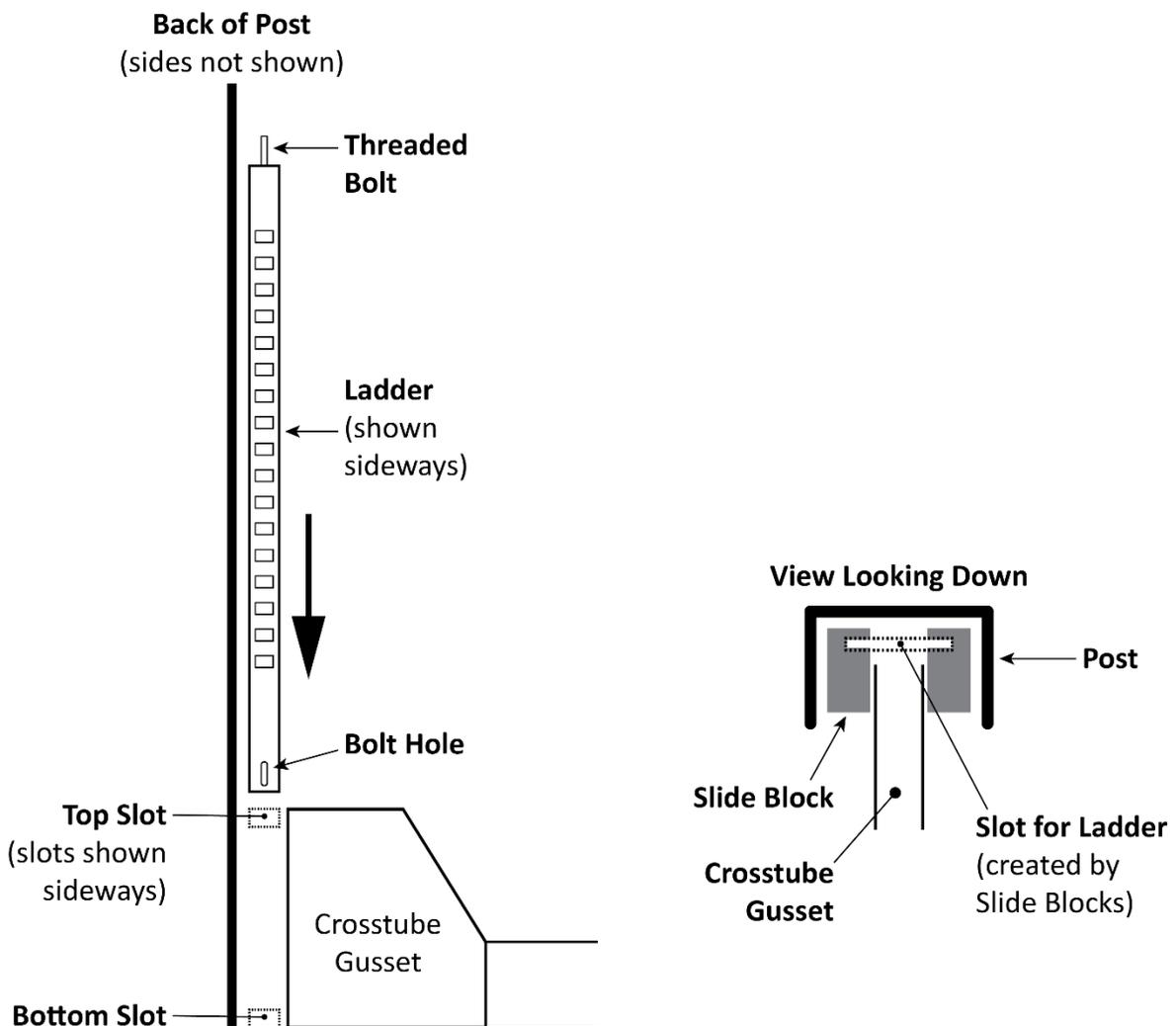
*Not to scale. Components removed for clarity. Front and side views combined. Make sure to install each Ladder through **both Slots** on each Crosstube Gusset.*
