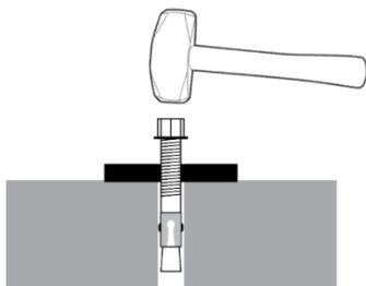
The Expansion Sleeve of the Anchor Bolt may prevent the Anchor Bolt from passing through the hole in the Base Plate too far; this is normal.
