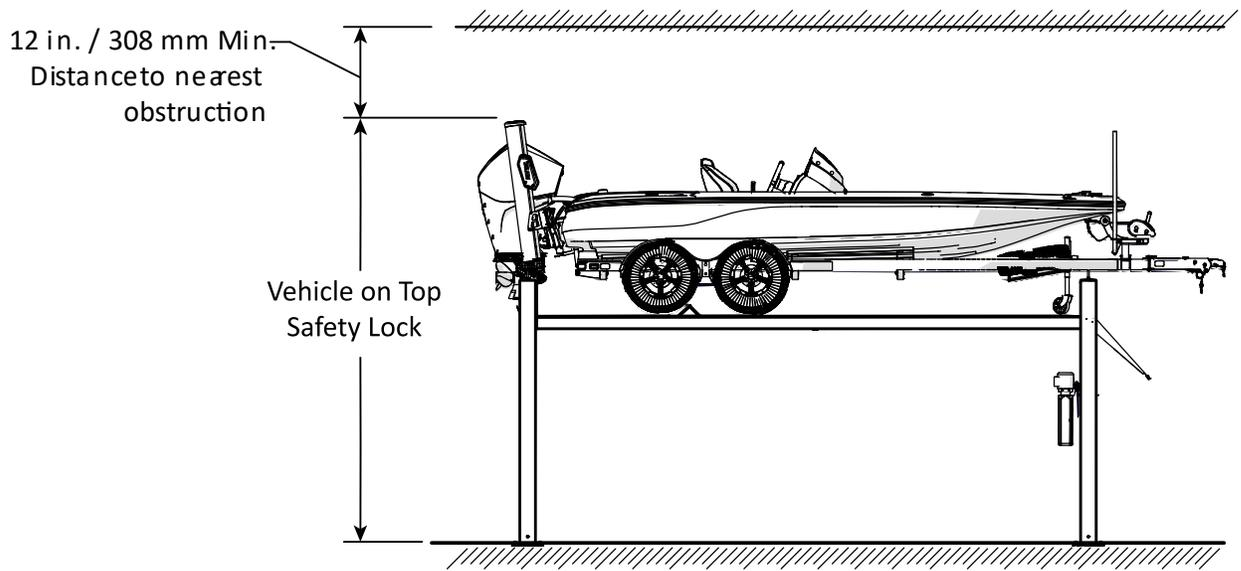
*Side view. Not to scale. Components removed for clarity.*
