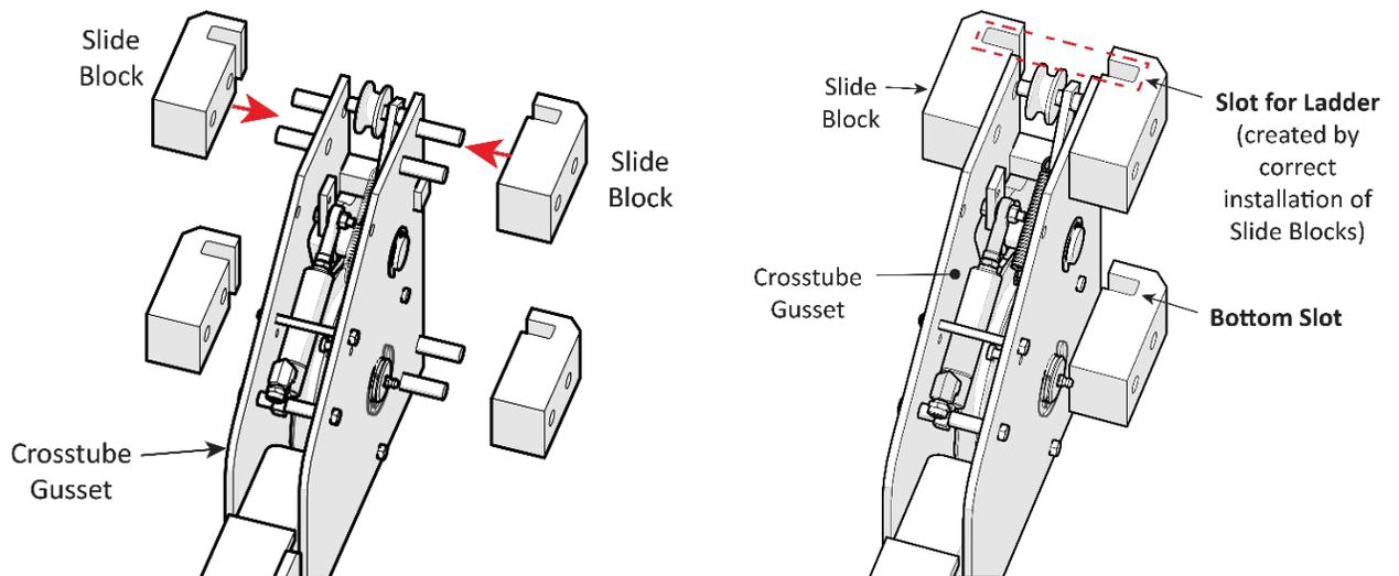
**Important:** It is easy to see the top Slot created by the Slide Blocks. It is difficult to see the bottom Slot, but it is **required** that the Ladder go through **both** Slots.
