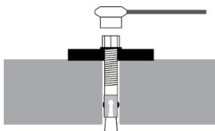
**Important:** Do **not** use an impact wrench to torque the Anchor Bolts.
