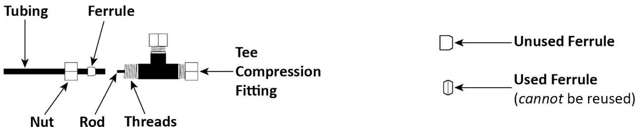
**Important:** **Ferrules can only be tightened once.** When you tighten the Nut on the Threads, the Ferrule is compressed; the Ferrule may not be reused after this compression.
