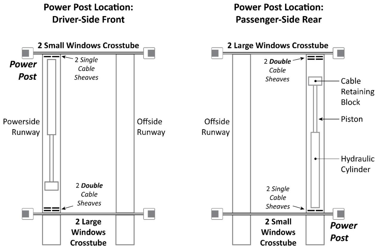
Top view. Drawing not to scale. Components removed for clarity. The location of the Ramps does not change based on Power Post location, but the Power Side Runway and Crosstube locations do. Windows are in the Crosstubes; they are shown here at the ends of the Power Side Runway for clarity.
