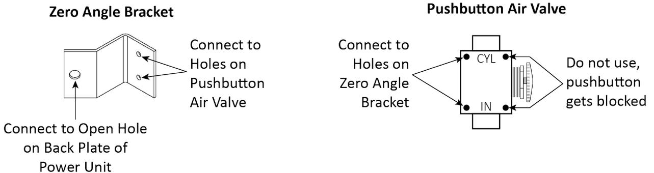
The following figure details the Pushbutton Air Valve and its connections.
