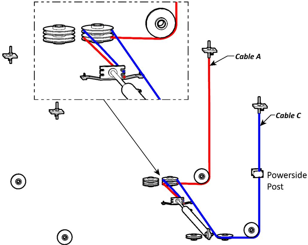
*Components removed for clarity. Not to scale.*
