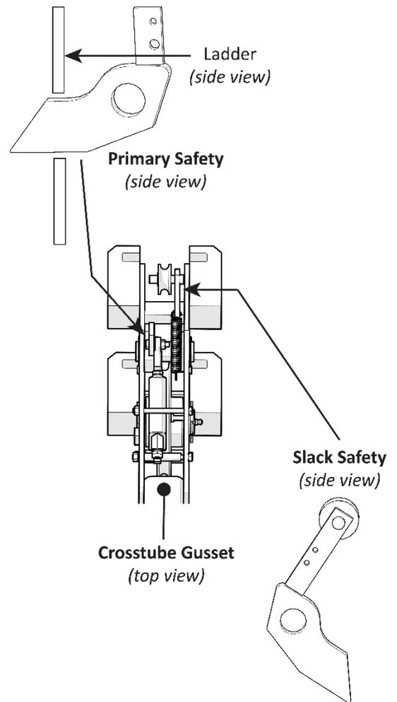
So how do the Runways come down if the Primary Safety Locks are engaged? To lower the Runways, you raise them a few inches (to get them off the Primary Safety Locks), then **press and hold down** the Pushbutton Air Valve. While you hold down the pushbutton, the Primary Safety Locks are moved away from the Safety Lock holes in the Ladders; they are prevented from engaging, which allows the Runways to be lowered.
