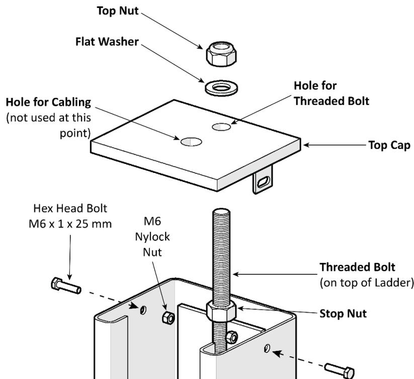
4. Put a Top Cap onto the top of the Post: put the Threaded Bolt on the top of the Ladder through the appropriate hole, put the tabs on the side of the Top Cap inside the Post, and secure the Top Cap on both sides with one Hex Head Bolt and one Nyloc Nut per side.
