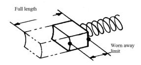
CARE: Worn brushes will result in power loss; cause the motor to run hot and irreparably damage the armature.
