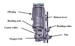
In the event that bending ann (roller) should fail to return automatically for any reasons (e.g. the bending arm (roller) has become jammed), turn the release lever to OPEN position. Make sure the release lever is in CLOSE position before resuming operation
