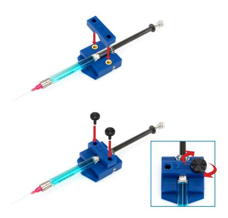
**5.10** Place the assembled syringe and clamp into the syringe pump cradle by sliding the "V" shaped bottom in (A), then push the syringe clamp toward the syringe pump cradle until it "pops" into place (B).
