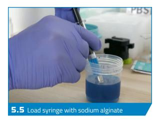
The syringe must be free of air bubbles in order to print successfully. If air bubbles are present, flip the needle upside down, put a finger over the tip, and pull back to create a vacuum. Then release your finger to move the bubble to the top of the syringe. Slowly compress the syringe until all of the air is pushed out, then proceed to fill the syringe normally.
