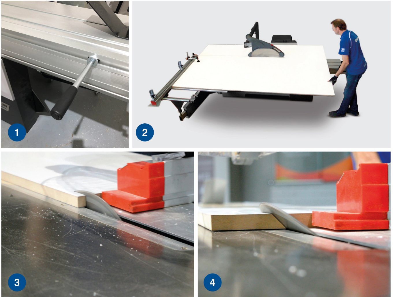
Fig. 1: Unlocking of the movable table.
