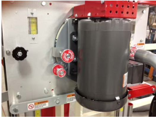
Figure 5: Proper Index Pin location for rip cutting (horizontal cutting).
