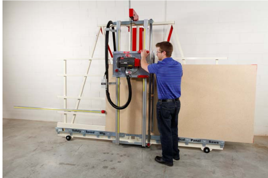
Figure 1: Crosscutting (work supported on at least two rollers). Model 7000 is used in the example.
