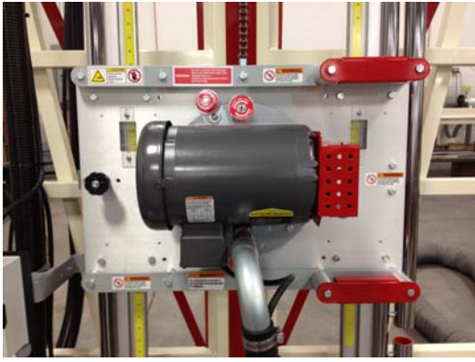
Figure 4: Proper Index Pin location for cross cutting (vertical cutting).
