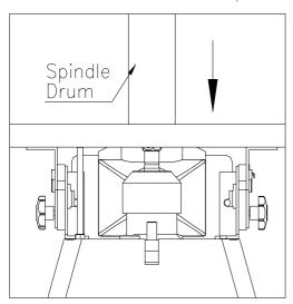
Fitting a new spindle drum.
