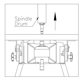
Removing an old spindle drum.
