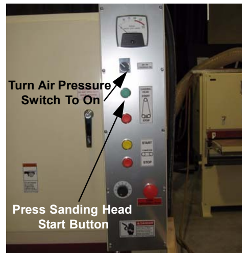
Figure 40: Air Pressure Switch and Sanding Head Start Button
