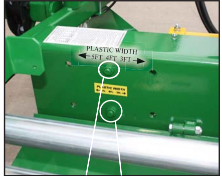
(No.2) Remove bolts on back side of bed former
