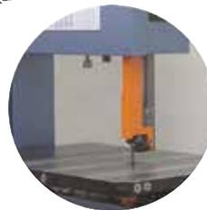
*26" throat depth is ideal for cutting large workpieces.*
