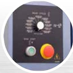
*Band speed control is conveniently located on the operator panel.*
