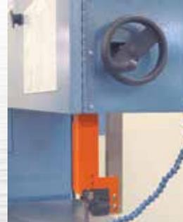
Post elevating handwheel
