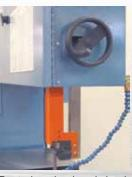
Post elevating handwheel
