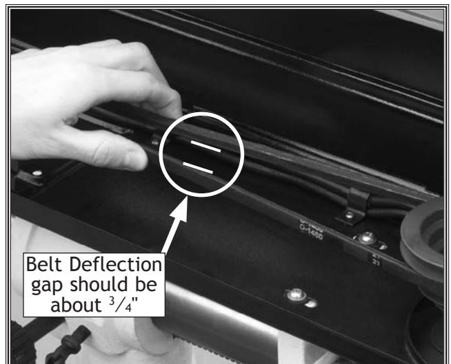
Figure 21. Measuring belt deflection.
