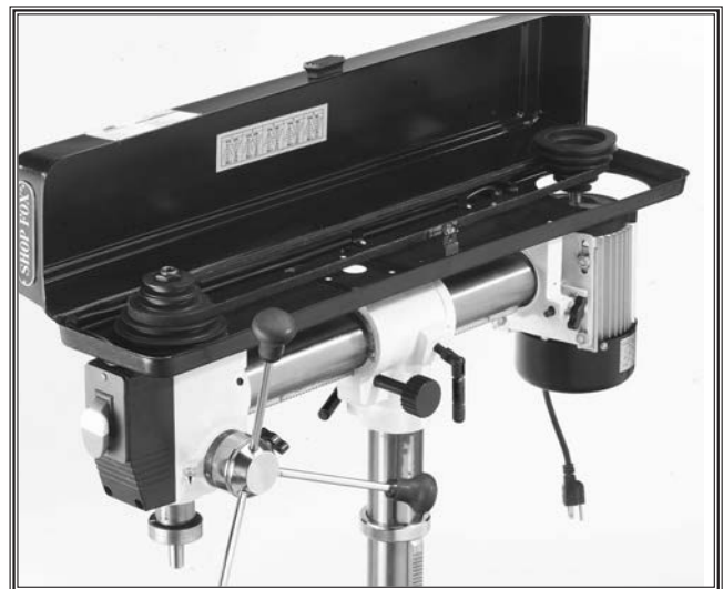
Figure 36. Adjusting belt to desired speed.
