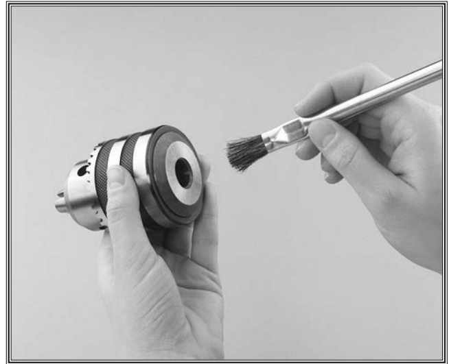
Figure 17. Clean the chuck before installation.
