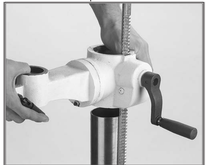
Figure 11. Installing rack and table bracket.
