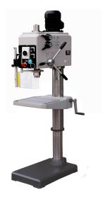
Clausing Production Series 230V Three Phase 19.7" GH Auto-Feed 1/1.5HP Floor Drill Press with Auto Reverse Tapping TLA25RS
