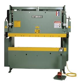
Betenbender 120 Ton 208V Three Phase 14' Bed Hydraulic Press Brake
