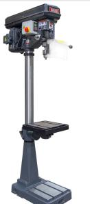
Dake Model SB-25 110V Single Phase 1" Drill Capacity Floor Model Drill Press 977600
