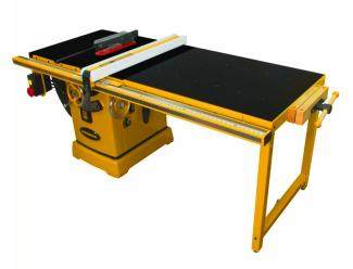
Powermatic PM2000T 10" ArmorGlide 460V Three Phase Table Saw with 50" Rip and Workbench Table PM9-PM25350WKT-4
