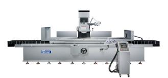
Sharp Industries 440V 20" x 47" SHT Series Traveling Column Surface Grinder SHT-2047-2A
