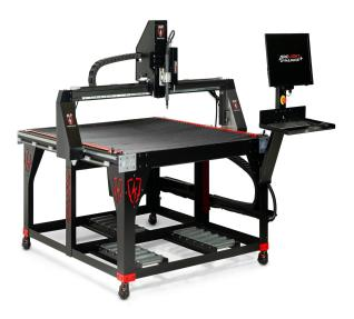
Arclight Arc Pro Ultra 5x5 CNC Plasma Table With 1" Thick Mild Steel Capacity
