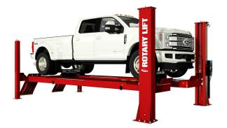
Rotary 4HP Single Phase 22,000 lbs. 309" Open Front Drive-On Alignment 4-Post Lift ARO22L
