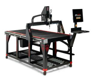
Arclight Arc Pro V2 Elite 4x8 CNC Plasma Table With 1.5" Thick Mild Steel Capacity and **Flashcut Control System**
