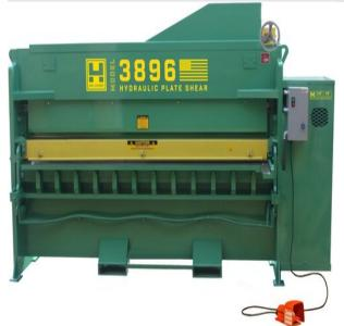
Uni-Hydro 7.5HP 220V Three Phase 0.375" x 96" Hydraulic Plate Shear 233896
