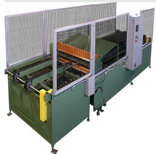
Ductformer 440V Three Phase 60" Fully Automatic Coil Line Wrap Brake DB-60
