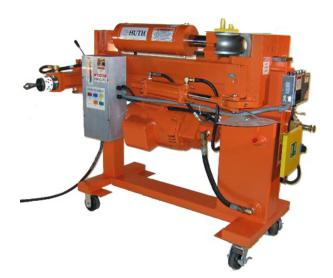
Huth 220V Single Phase 7.5HP Manual Knee Control Heavy Duty Horizontal Pipe Bender 2601HD
