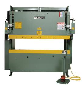
Betenbender 160 Ton 460V Three Phase 8' Bed Hydraulic Press Brake
