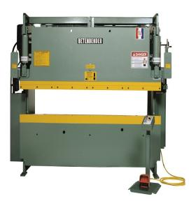
Betenbender 160 Ton 460V Three Phase 10' Bed Hydraulic Press Brake
