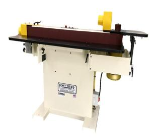
Ritter Machinery 480V Three Phase Oscillating Double Sided Horizontal Edge Belt Sander R933
