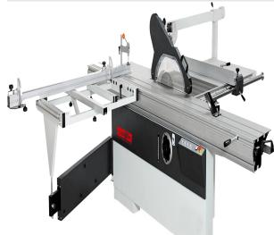
Cantek 5 HP Single Phase 10' Sliding Table Saw with Scoring P305
