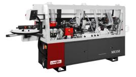
Cantek 230V Three Phase 29FPM Automatic Pre-Milling Compact Edgebander with Quick-Change Glue Pot MX350
