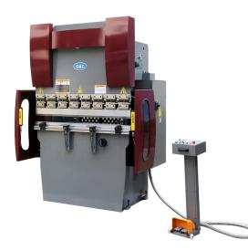
GMC Machinery 7.5HP 220V Three Phase 33 Ton 5ft CNC Hydraulic Press Brake with Estun Control HPB-3305
