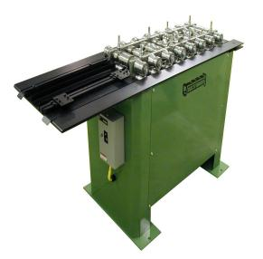
Ductformer 5HP 480V Three Phase Rollformer CR8
