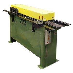
Ductformer 7.5HP 220V Three Phase 18-26 Ga 14 Station TDFC Rollformer CR14-TDFC
