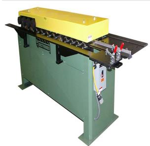
Ductformer 7.5HP 220V Three Phase 18-26 Ga 12 Station TDFC Rollformer CR12-TDFC
